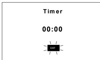
Key in the time required in minutes and seconds using the numerical keys, then press [OK] to start the timer. The maximum time is 29 minutes and 59 seconds. Use the  $\leftarrow$  and  $\rightarrow$  keys to reposition the cursor and re-enter the time if it is keyed in incorrectly.
