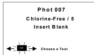
Place a BLANK TUBE in the test chamber, then press [OK].
