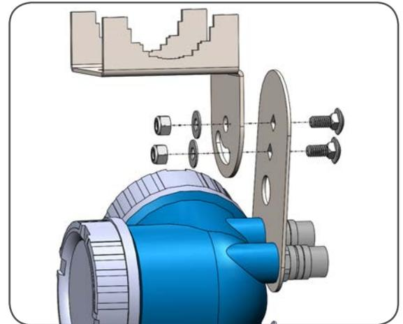
Mount Pole Bracket to Flange Plate
