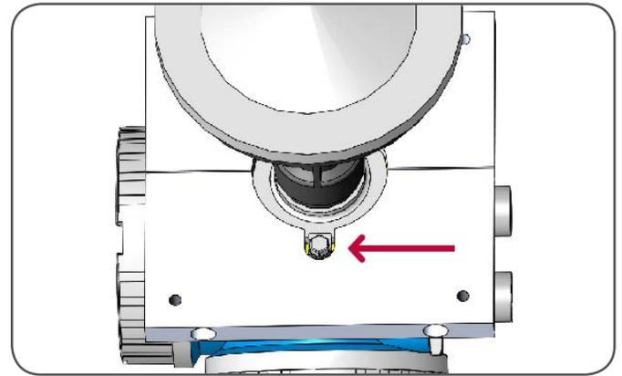
Align Cut-out in Flange to Radar Retaining Clip
