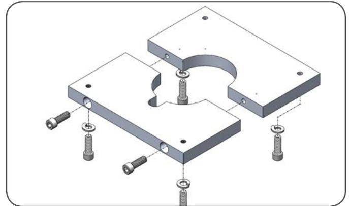
Nile Radar Sensor Mounting Flange Kit
