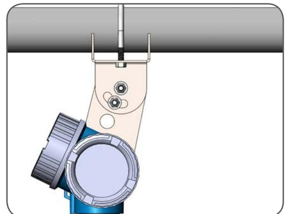
Mount Radar and Bracket on Pole, and Align the Radar Unit for Optimal Radar Function
