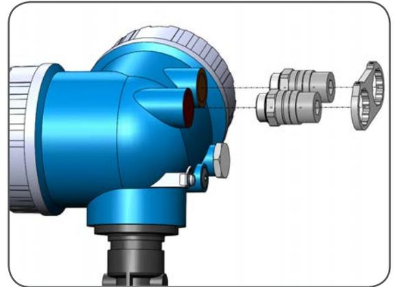
Remove Wire Nut Retaining Bracket and the two Wire Routing Nuts
