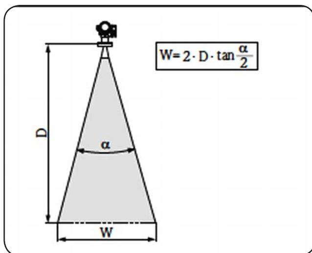
*Relationship between beam angle  $\alpha$ , distance  $D$ , and beam width diameter*
