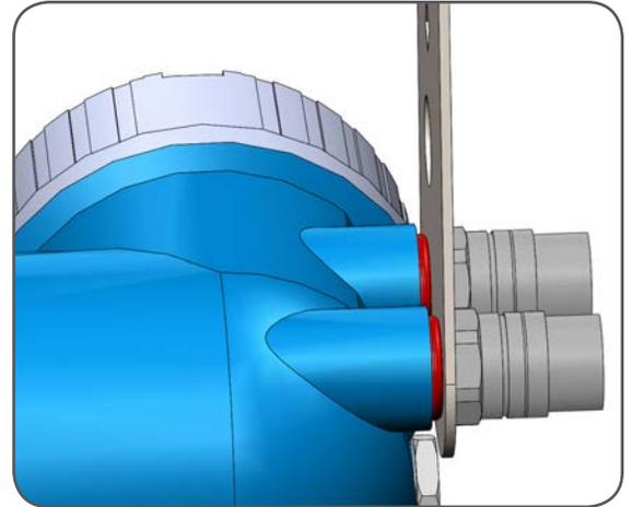
Reinstall Wire Routing Nuts
