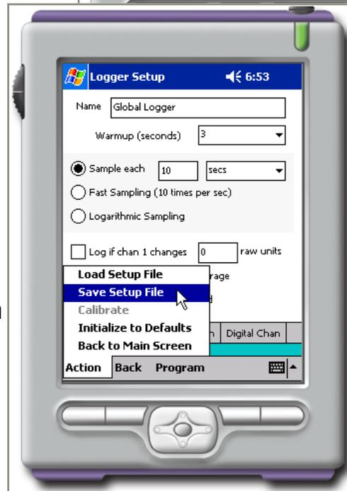
Initialize to defaults restores the logger to default factory settings. It is recommended that this function not be used and a warning will occur before settings are changed. Using this function does not reprogram the logger but rather, just changes the information in the setup screens.
