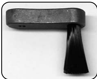
Level 1- New brush, minimal "splay"
