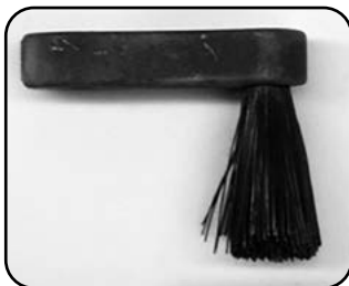
Level 2- Moderate splaying, have spare ready
