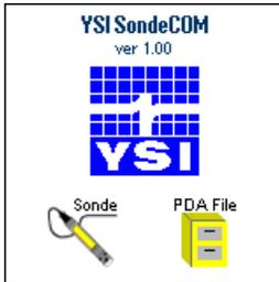
Every time you launch SondeCom, you will see this startup screen. There are only two buttons on this screen: the *Sonde* button and the *PDA File* button. If you press the *Sonde* button, then SondeCom will try to establish a connection with your 6-Series sonde. If the connection is successful, then you will be in the sonde menu.
