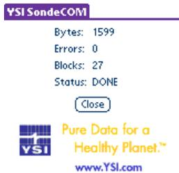
To upload a file from a sonde to your PDA, simply navigate through the sonde menu (File | Upload or File | Quick Upload) to the upload data option. SondeCom will automatically handle the Kermit data transfer. Once the transfer has completed, tap the close button to return to the [sonde menu](#).
