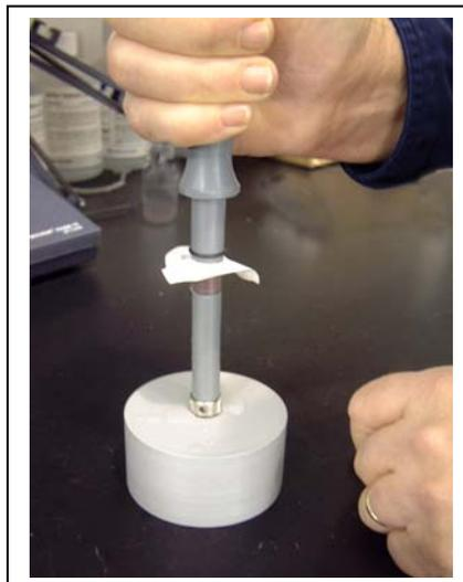
As shown in the picture below left, roll the o-ring off of the end of the installation tool so that it resides in the o-ring groove of the probe. Be sure to hold onto the O-ring prior to removing the installation tool so that it does not pop out of the groove. Then, as shown below right, remove the installation tool and make certain that the o-ring is centered in the groove on probe end.
