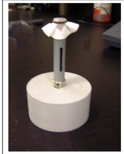
As shown in the picture below, use a razor blade or knife to trim away the excess membrane material.
