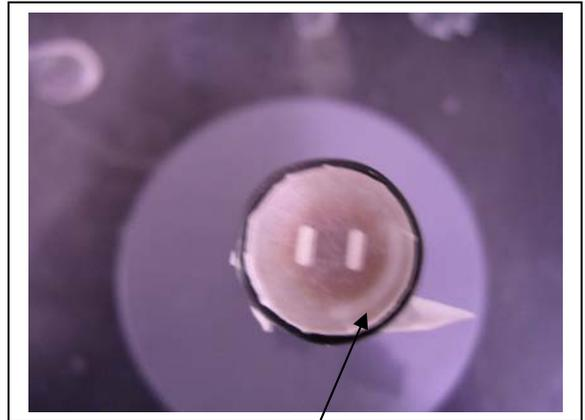
**Note the presence of a bubble after installation. This is acceptable for a free chlorine membrane.**
