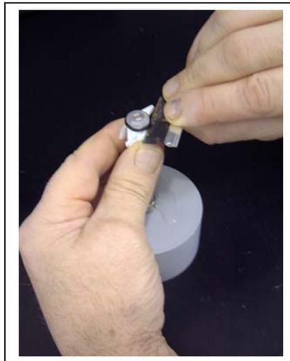
The pictures below show a properly installed free chlorine membrane. Note that, because the membrane will not stretch, there may be some points where the membrane is slightly “bunched up” in the o-ring groove. This effect is normal and will not affect sensor function. Also note that the presence of bubbles under the membrane is also normal and should not affect probe function.
