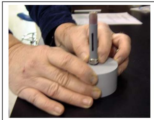
Place an o-ring from the 6573 membrane kit in the groove at the bottom of the tool as shown in the picture below left.
