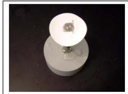
As shown in the picture below, place the bottom of the o-ring installation tool over membrane/probe face and press down securely.
