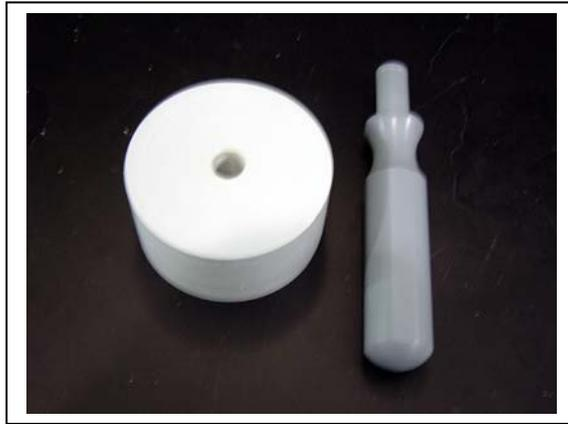
Thread the nut on the end of the 6572 probe into the base plate as shown in the picture below.
