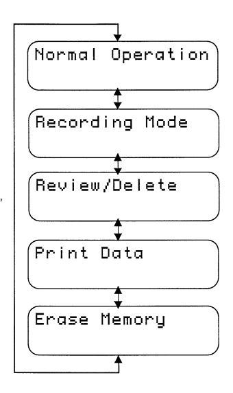
To activate the Memory feature of the YSI Model 59, press the  $\leftarrow$  key while the function switch is set to  $O_2$ -TEMP. A display similar to the following will appear:
