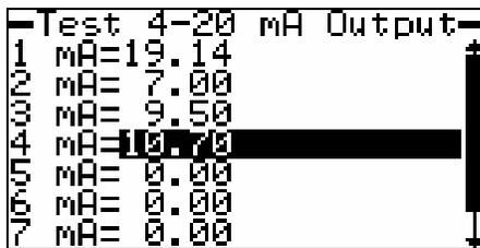
Alternatively, you may highlight particular loops, one at a time, (e.g., loop 4 shown above), then enter a value of your choice. One approach is to test each loop output using 4, 12, and 20 mA signals to simulate the 0%, 50% and 100% scale of the specific parameter assigned to that loop. Then follow the procedure above to test the mA values at the input of the SCADA.
