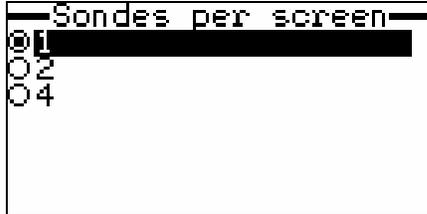
If you have more than one sonde connected, you can choose to view 1,2, or 4 sondes per screen. Highlight the desired setting and press Enter to select it. If you choose “1 sonde/screen”, you can still view the data by scrolling right and left to view the other sondes connected. If you have three sondes connected, you can choose “4 sondes/screen” to view all of the sondes on the screen. One section will appear blank.
