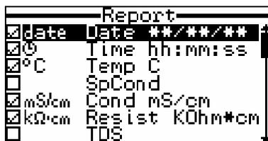
The Report menu allows the user to configure the 6500 display readouts. A list of the possible parameters and the currently selected units for each parameter will appear. The user can select a displayed parameter using the  $\uparrow\downarrow$  arrows to highlight. When the desired parameter is highlighted, the user can press Enter to display the Select Units menu for the specified parameter. The following screen will be displayed.
