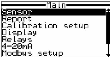
Use the ↑↓ arrow keys to highlight the submenu options. Press Enter to select a highlighted option.
