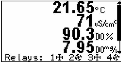
If a relay is active, the symbol will be spinning as is simulated above for relays 2 and 4. If the relay is inactive, the symbols will be stationary as shown above for relays 1 and 3.
