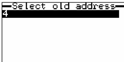
To change an SDI-12 addresses, highlight the current SDI-12 address of the sonde you wish to change and press Enter to select it. A new screen showing available new addresses will be displayed.
