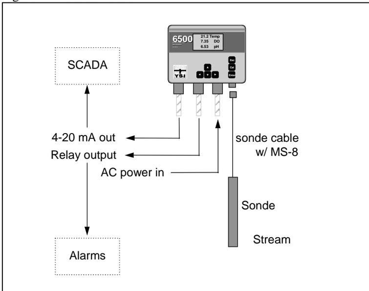
Figure 5 Sonde installed distant from the 6500 Monitor
