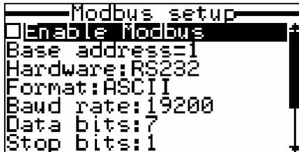
Use the arrow keys to highlight **Base address** and press Enter to select it. This will activate a cursor which is used to change the 6500 Modbus base address. To increment the address, use the ↑↓ arrow keys. When the desired address is reached, press Enter to set it.
