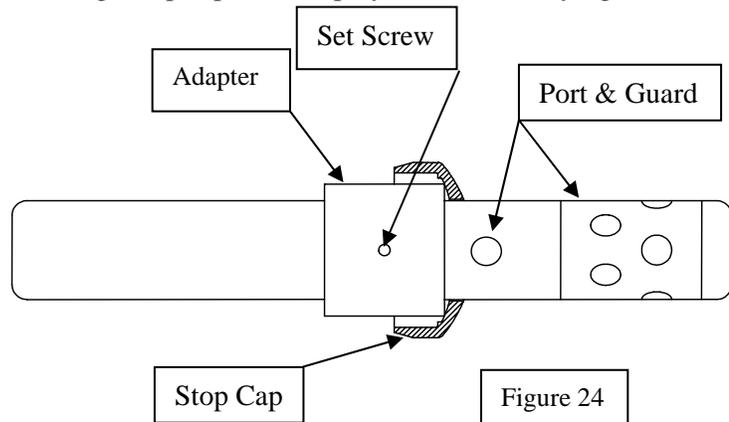
2. Attach the stop cap to the end of the PVC pipe using PVC cement, as per instructions on cement can label, ensuring that the stop cap is positioned straight and the pipe is fully inserted.
