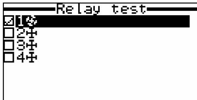
If the above test is positive, the alarm (light, siren, etc.) should activate if the 6500 Monitor is functioning properly. If no activation occurs, contact customer service for advice. If the alarm does activate, press Esc to return to the “Relays” menu, then highlight the “Configure” relays selection and press Enter.
