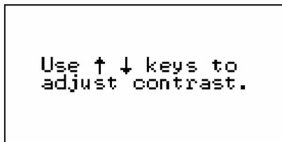
Using the  $\uparrow\downarrow$  arrows, select the desired screen contrast. Then press Esc to return to the Display menu.
