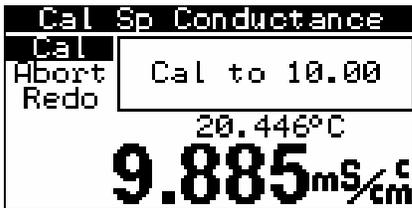
This display allows you to view in REAL TIME the actual specific conductance values from your probe. At this point you also have the option of aborting the calibration completely to return to the Run display by highlighting the Abort selection and pressing Enter. If you inadvertently entered the wrong value for your standard, highlight Redo and press Enter. You may reenter your numerical calibration value at this point.
