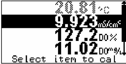
Use the arrow keys to highlight the output line for specific conductance as shown above. Press Enter and the following display will be shown.
