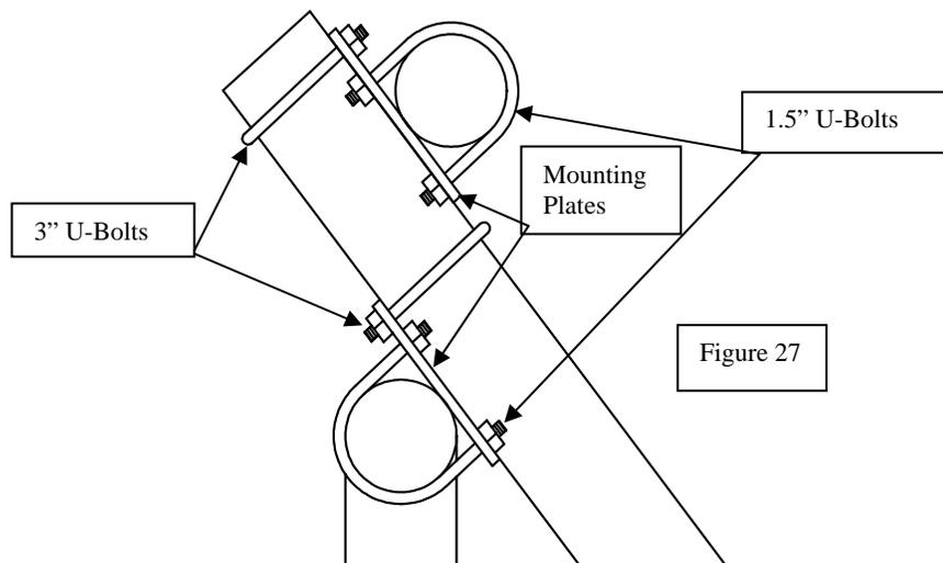
2. Loosely fasten two 1-1/2" u-bolts on each mounting plate to the railing, orientated as shown in Figure 27.
