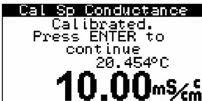
Now simply press the Enter key to return to the Calibration display and proceed to calibration of the other sensors using the same basic procedures as described above for specific conductance.
