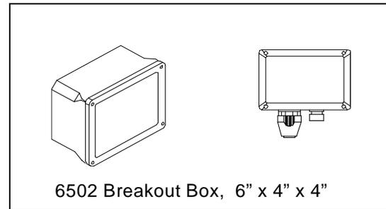
The Breakout Box may be mounted on a wall or to a vertical pipe or handrail that is 1 to 1½ inches in diameter. Rail mounting the 6502 Breakout Box requires the optional the 6509 Rail Mounting Kit. The location of the 6502 Breakout Box should be elevated and in a dry place above potential flood level. The Breakout Box should be easily accessible for an operator or technician.
