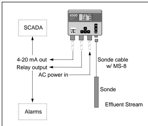
System set-up, including calibration of the 6-Series Sonde sensors, can be performed at the site with the 6500 Monitor front panel keys and LCD or in the laboratory with a personal computer or a YSI 610 Display/Logger.
