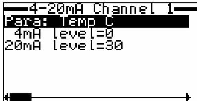
First, choose the parameter which will be associated with the selected 4-20 mA channel by highlighting the “Para:” selection and pressing Enter to display a list of available parameters. Using the up and down arrow keys, select the desired parameter and then press Enter to confirm the selection (temperature in degrees Celsius in the example).
