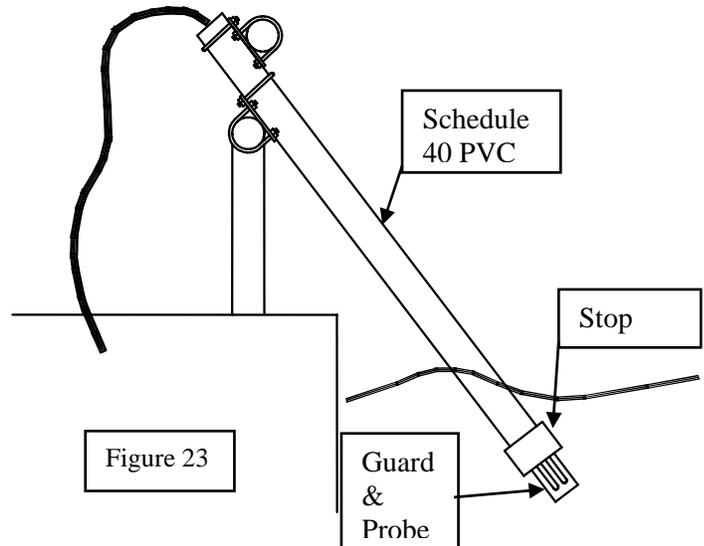
The 6511 Kit should not be mounted on hot or vibrating pipes or structures, or near high heat sources, AC motors or transformers, radio transmitters or antennas.
