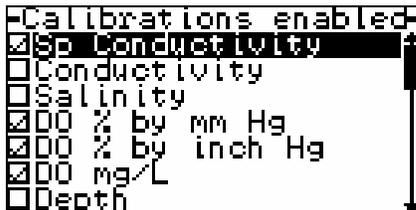
Once a calibration is selected as indicated by the check mark, that sensor may be calibrated using the Cal key during the Run mode. The user can select and deselect items using the  $\uparrow\downarrow$  arrows to highlight and press Enter to toggle selections on and off.
