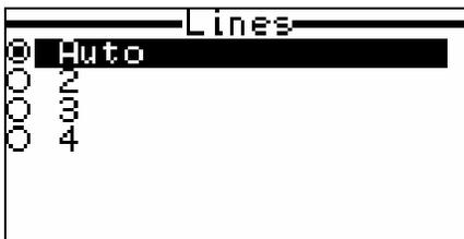
Four selections are possible from the Display setup menu: Auto, 2, 3 and 4 lines per screen. Highlight the desired item with the up and down arrow keys and press Enter to toggle it on. Only one choice is allowed.
