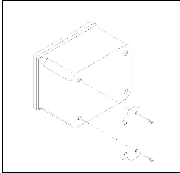
4. Tighten the screws, securing the Monitor to the surface.
