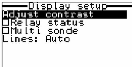
The Display menu contains options concerning the visual display of the 6500 Monitor. Use the  $\uparrow\downarrow$  arrows to highlight the desired display feature. Press Enter to select the feature.
