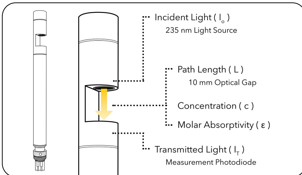
The concentration of nitrate ions,  $\text{NO}_3^-$  mg/L, is proportional to the optical absorbance of the UV-C radiation. It is important to note, however, that the UV method presented by YSI does not distinguish between nitrate  $\text{NO}_3^-$  and nitrite,  $\text{NO}_2^-$ , owing to similar UV absorption properties and we therefore denote the combined species,  $\text{NO}_3\text{-N}$  (nitrate as nitrogen). However, in natural waters, nitrate is typically the most prevalent species.
