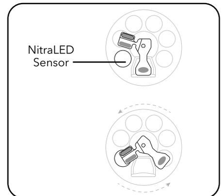
(Top view) Center Wiper Arm within NitraLED Sensor window
