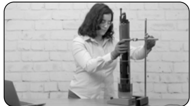
Place the sonde into the beaker of raw water and hold in place with the ring stand clamp. Verify that the entire colored part of the NitraLED sensor and the Turbidity sensor are submerged.
