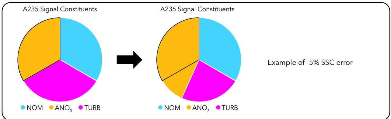
With a positive 5% error in the SSC coefficients, the effect of turbidity and NOM interference is overestimated, resulting in an underestimation of nitrate. With a negative 5% error in the SSC coefficients, nitrate is overestimated.
