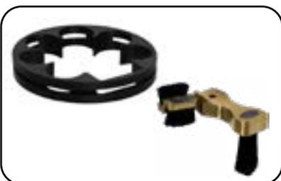
The **EXO Alignment Ring** fits around the EXO sensor payload to minimize movement while the NitraLED Wiper Brush cleans the sensor faces. The Alignment Ring is held tightly in place by an o-ring that makes contact with the sensors. A **NitraLED-specific wiper** effectively cleans all sensor faces with its two-arm design.
