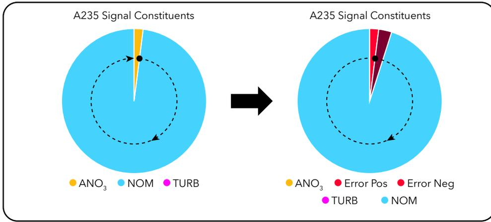
In this case, with the same +5% overestimate for the NOM coefficient, the nitrate estimate is now consumed by the error resulting in negative NitraLED readings.
