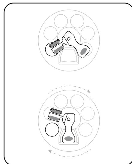
Rotate back so the main brush is over the guard.
