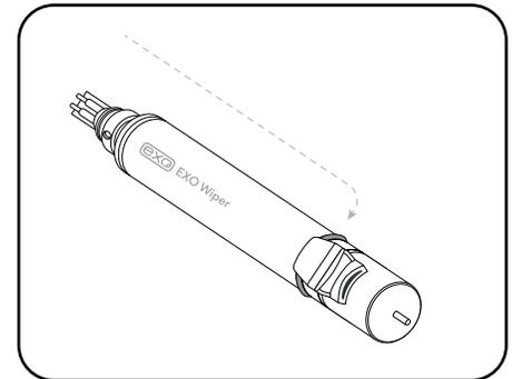
3 Install the Central Wiper on to the sonde bulkhead.
