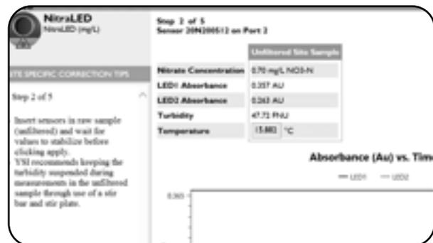
If this option is selected from the Step 2 screen, the user will be directed to Step 4 after a measurement has been taken in the raw sample water. The software will then indicate that the sensor should be placed into the filtered water sample
