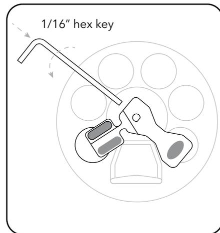
Tighten screw on back of Brush while centered in Nitrate window.
