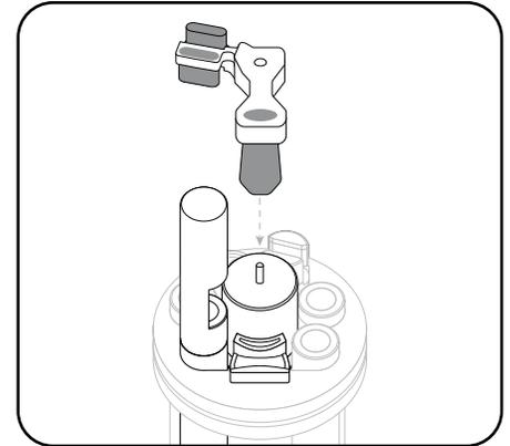
Slide Brush down until fully seated on top of the Central Wiper
