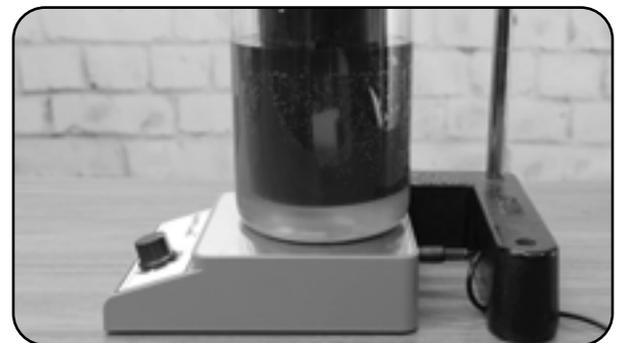
**NOTE:** While the sensor LED values are stabilizing, verify that there are no bubbles accumulating on the sensor faces of the NitraLED or turbidity sensors. Be sure to watch the turbidity values for stabilization as well. If turbidity continually rises over time, this is most likely due to bubbles accumulating on the sensor face. Even the smallest bubbles can have an impact on sensor readings; if there are bubbles, remove the sonde from the water briefly and reinstall.
