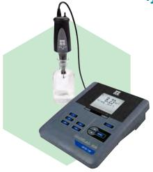
As the direct replacement for the YSI 5000, the MultiLab 4010-1W is most often used in water resource recovery facilities (WRRF) for the determination of biochemical oxygen demand (BOD). A typical 4010-1W configuration includes:
