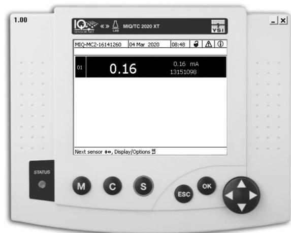
Figure 1: Press the "S" button on the IQ SensorNet controller
