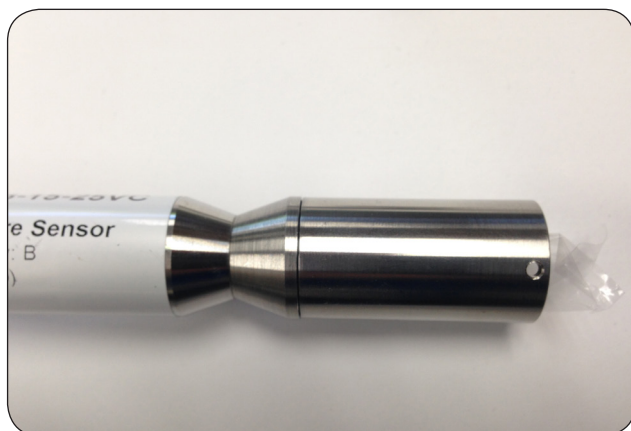
Install the Protective Housing over the Media Barrier Bag and O-Ring
