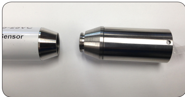
Screw the mount into the end of the H-3123
