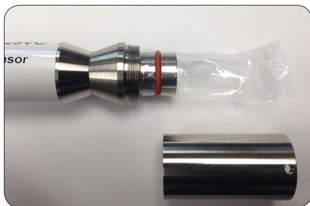
Install the Media Barrier Bag into the H-3123
