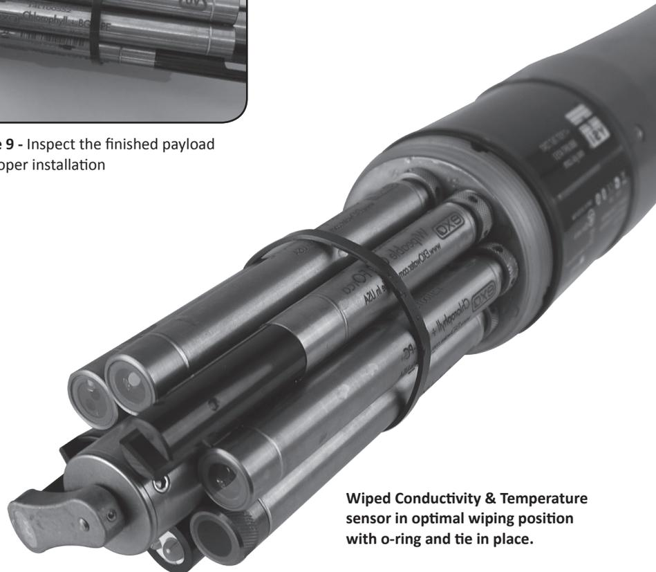
**Wiped Conductivity & Temperature sensor in optimal wiping position with o-ring and tie in place.**
