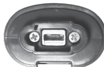
Bottom view: micro USB connector with rubber cap open.
