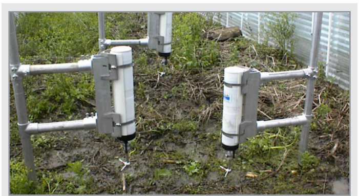
A flume built for a study on nutrient uptake shelters. Three ADVs study the movement of water and sediment through Louisiana's Caernarvon Diversion. Pulse-coherent technology offers highly accurate readings even in extremely shallow or slow-moving water.
