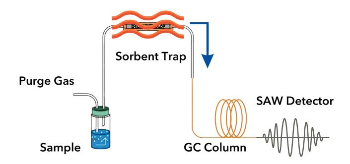
YSI's new THM Analyzer is an easy to operate, integrated Purge & Trap Gas Chromatograph (GC) that measures THM concentration at ppb levels in less than 30 minutes right at your own facility with a simple walk up and run protocol. This integrated system is a powerful new tool that can help operators optimize water treatment at the plant and evaluate water age in the distribution system for improved control over the formation of THMs.
