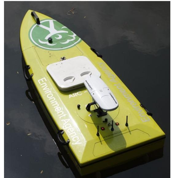
ARC remote control boat in operation.
