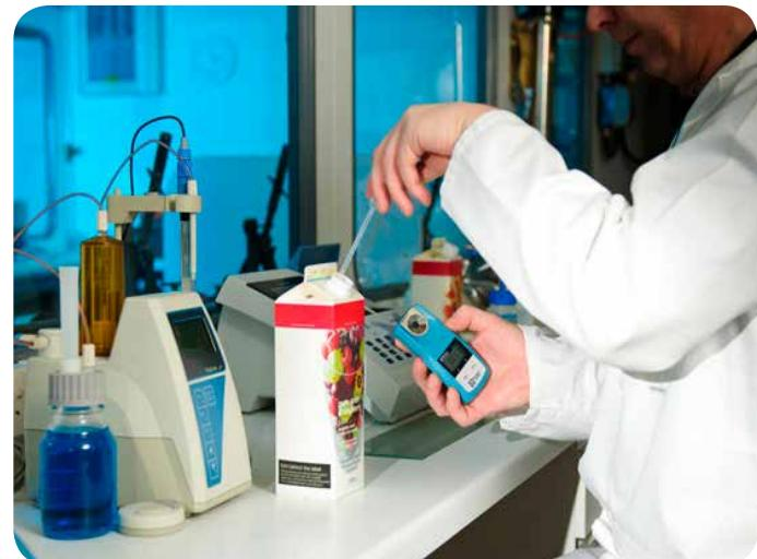
Fig. 7: OPTi digital handheld refractometers have temperature compensation so that Brix readings are consistent in the factory, laboratory or in the field.
