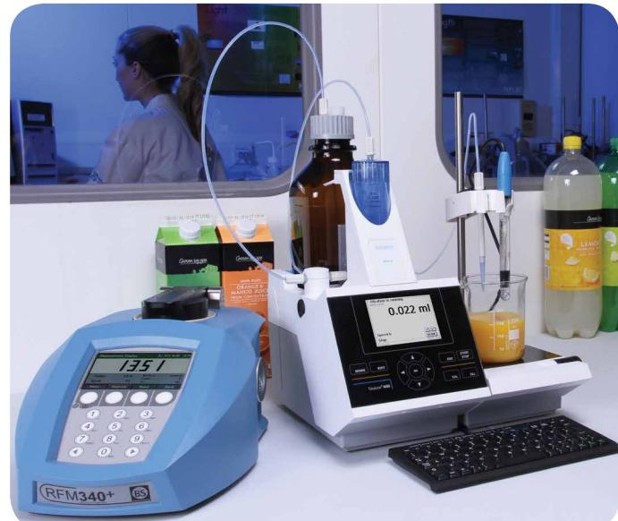
Fig. 1: The popular RFM340+ Series Peltier temperature controlled refractometer (left) used to control Brix in the factory or laboratory next to a TitroLine 7000 auto-titrator (right) for controlling acids and diet beverage concentrations
