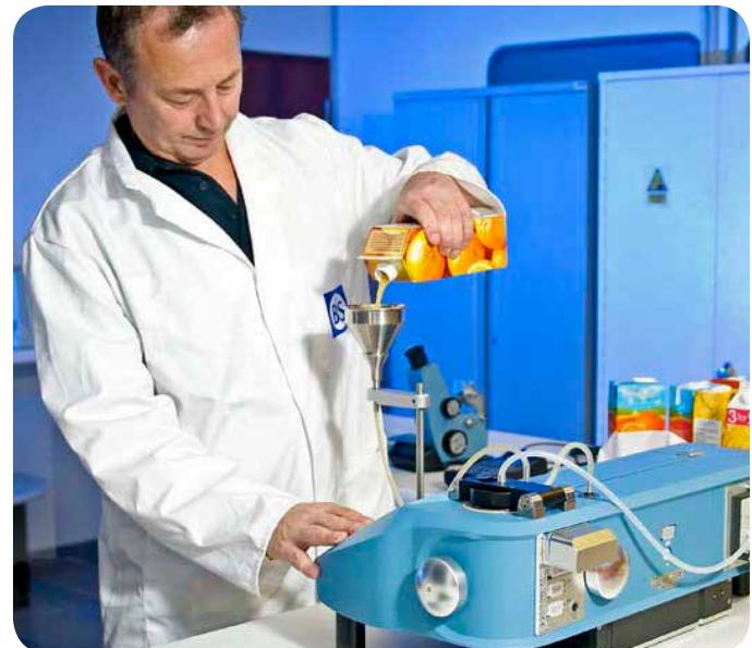
Fig. 8: The Pro-Juice refractometer pre-conditions orange juice samples so that lines can run just above the lower threshold of product filling specification providing optimum yield from concentrates and thus helping to improve profitability from reduced waste or "over Brixing."
