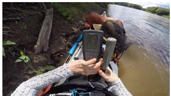
Pohl preparing to take Specific Conductance, TDS, and Dissolved Oxygen measurements with the YSI Pro2030.
