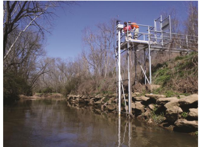
Technicians remain dry and safe while accessing instruments from a stable stormwater monitoring platform.
