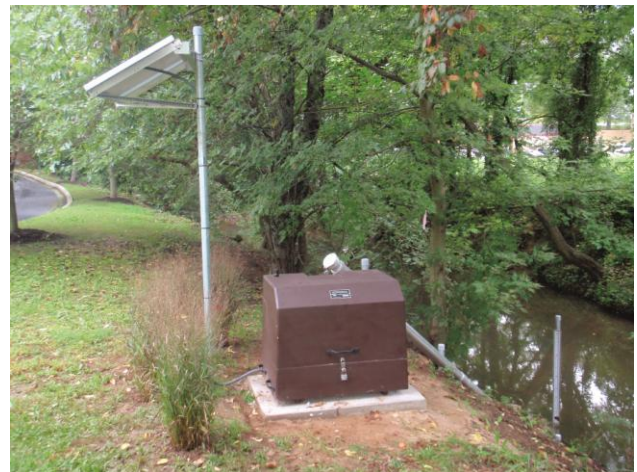
Temporary stormwater monitoring platforms collect data for short-term studies and can be moved throughout a watershed.
