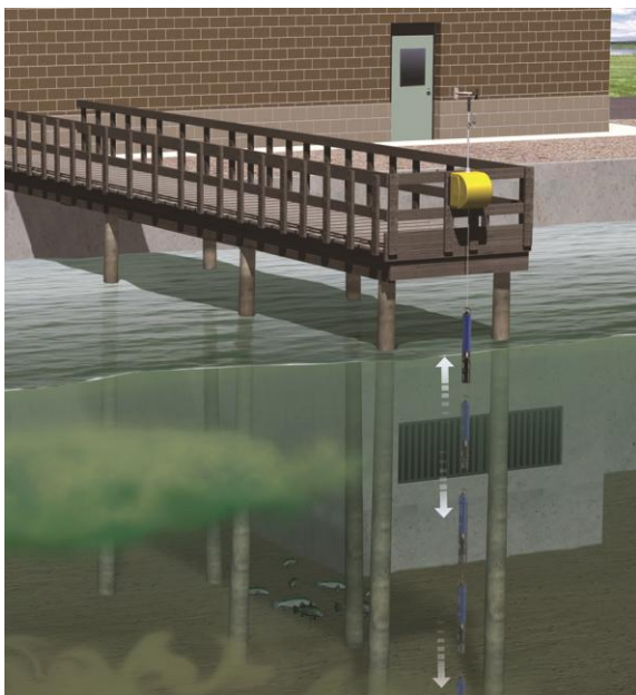
The Total Algae sensor on the EXO sonde moves up and down, profiling the water column, and can detect subsurface algal blooms.
