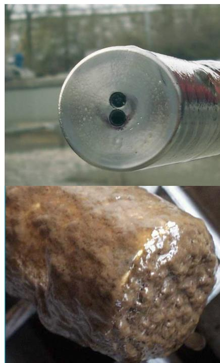
Optical sensors for turbidity and suspended solids measurement are ideal for wastewater applications. The VisoTurb® turbidity sensor is shown here after a 30 day continuous deployment. The top image shows the sensor with ultrasonic cleaning and the bottom image was in the same setting without the cleaning system activated.
