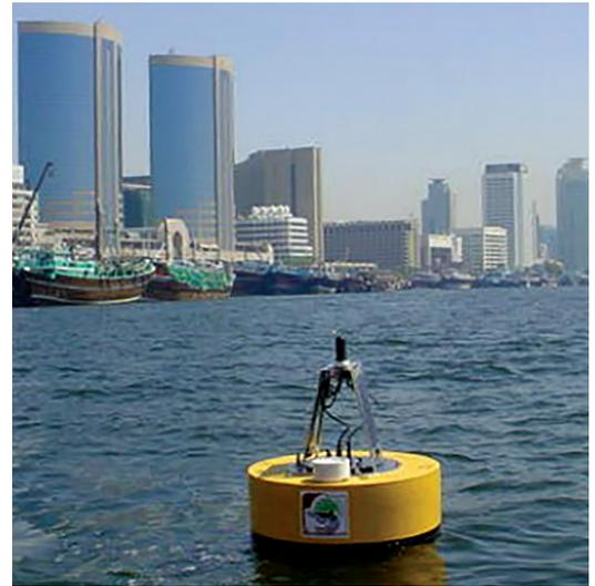
YSI Water Quality Monitoring Buoy on Dubai Creek
