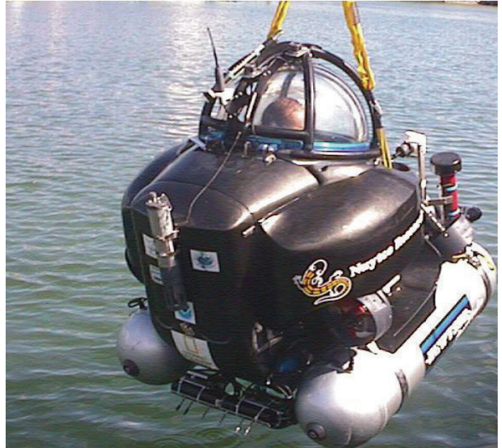
An SSE DeepWorker 2000 submersible vehicle with a YSI 6600 Multiparameter sonde.
