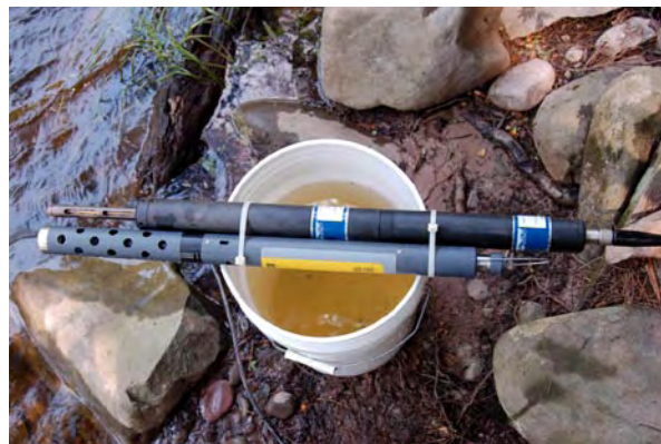
Simultaneous field trial of ROX sensor and DO sensor from alternate company
