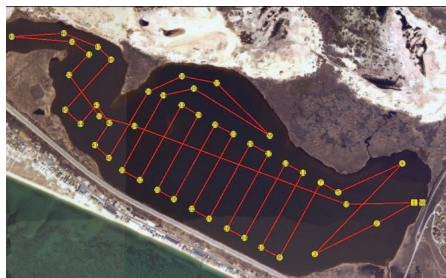
Screenshot from VectorMap mission planning software showing a "lawnmower"-style mission path drawn onto image of saltwater lagoon.
