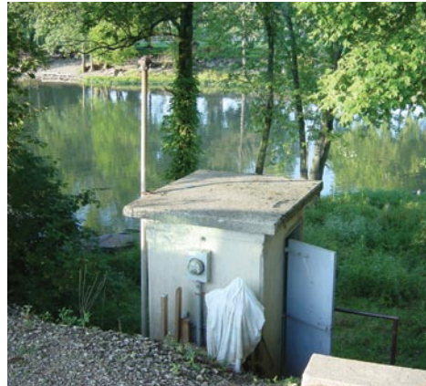
Figure 1a. Typical gage station for sidestream monitoring of rivers, during normal flow.
