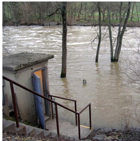
Figure 1b. Gage station at high flow/high turbidity. Sidestream methodology prevents the water quality sensors from getting damaged during flood events.
