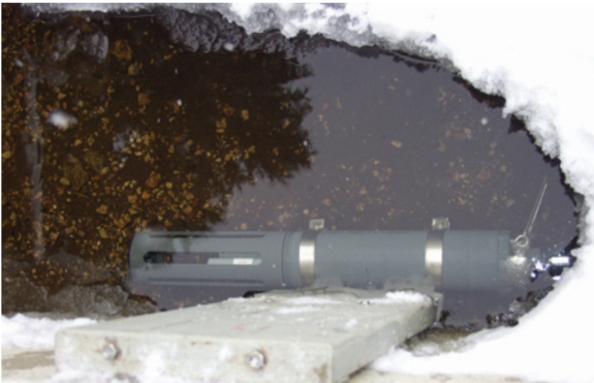
YSI multiparameter sonde deployed under the ice.
