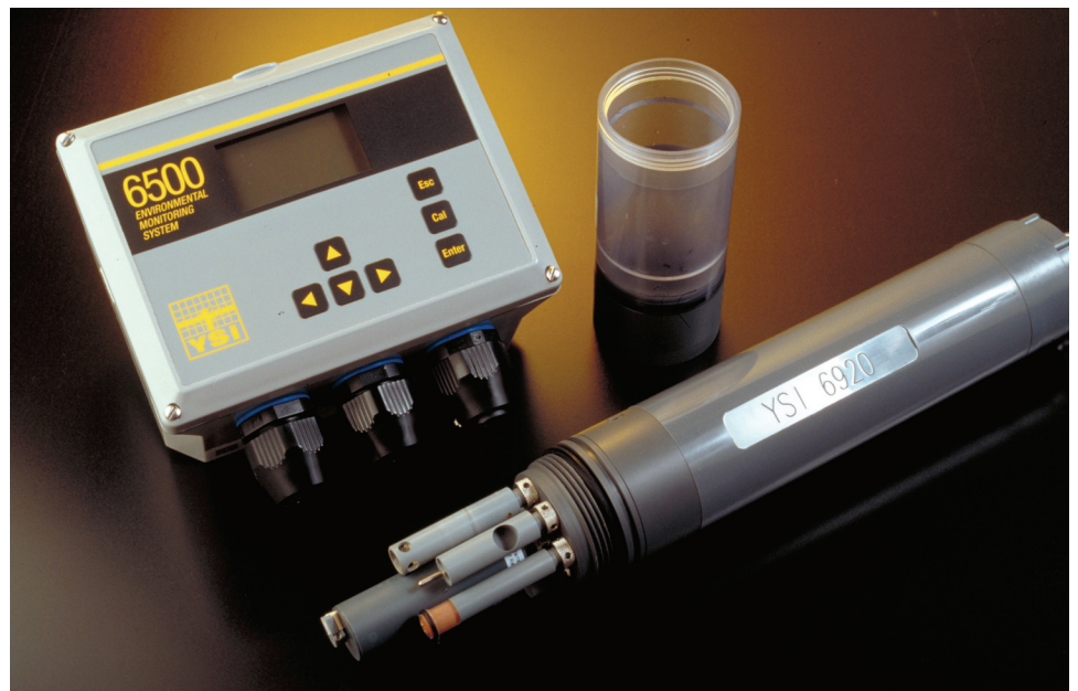
YSI 6500 Environmental Process Monitor with a YSI 6920 Multiparameter sonde.
