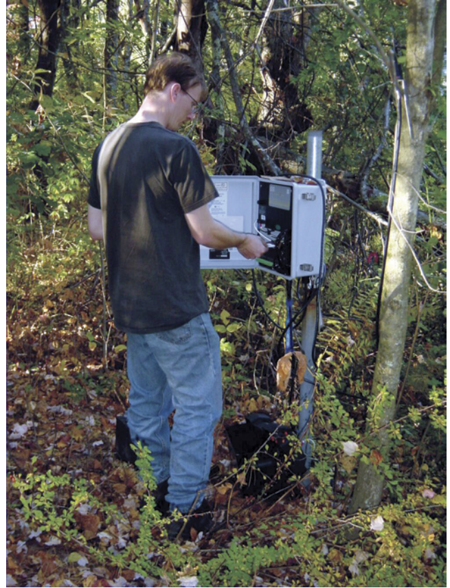
IPSWATCH field technician with a YSI 6200 DAS.
