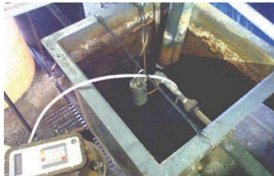
YSI 6920 deployed at a metal coating/metal anodizing industrial waste pretreatment site.
